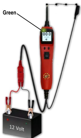
Continuity (less than approx. 650 \Omega )
