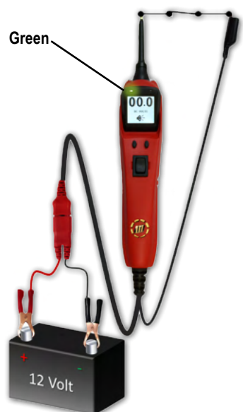
Continuity (less than approx. 650 \Omega )
